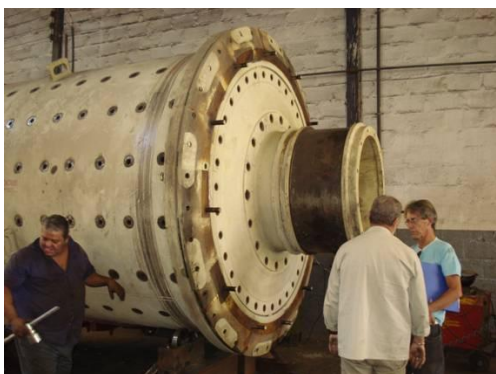
Figure 5 – Second hand ball mill being refurbished
